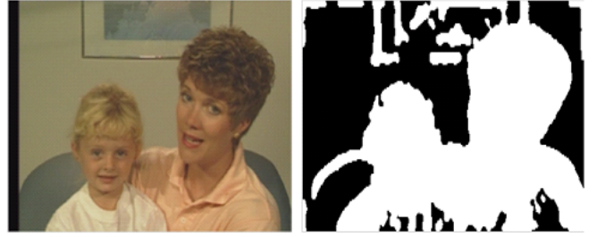
Fig. 3. Mother video (left) and the detected saliency (right) after thresholding by B=4\% of the bit depth.
